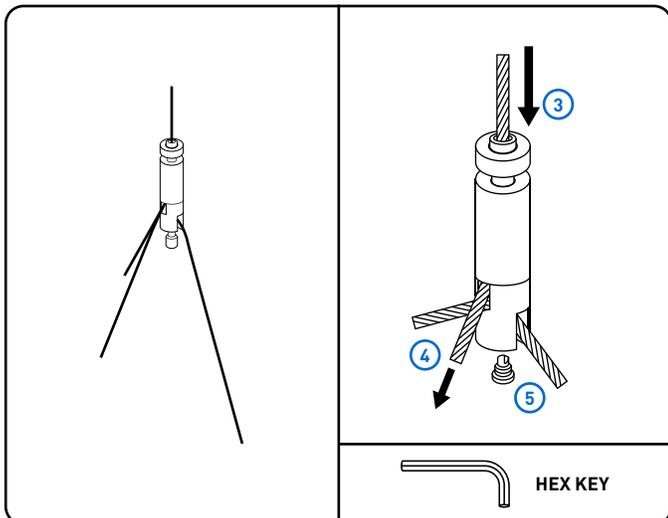
3) Insert the suspended vertical cable end into the adjustable suspension fitting on the sling cable.
