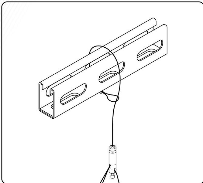
2) Attach the clip hook sling to the luminaire frame.
